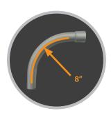
DigiTemp is small enough to easily deploy through standard 1" (2.5cm) PVC conduit with 8" (20.3cm) factory bend corners.
