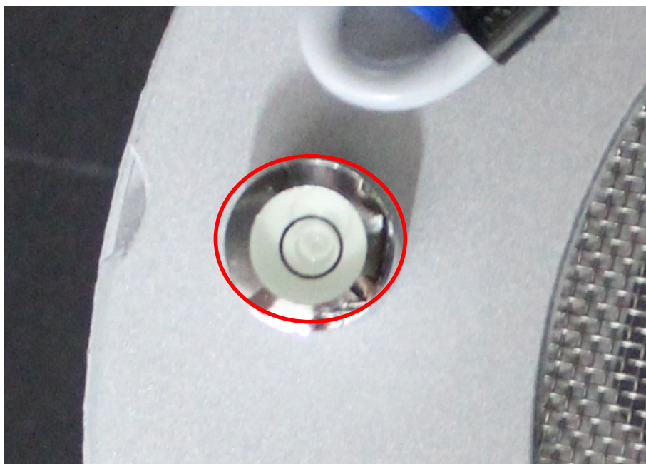
Figure 6: Leveling of set up during installation (close-up view)
