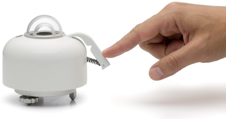
Figure 4.2.2 Installation of sun[e]'s sun screen
