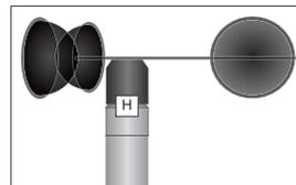
Under most climatological conditions the heating prevents blocking of the moving sensor parts (see illustration). The cup rotor or the wind vane are not heated. In case of icing or formation of ice at the moving sensor element the function is restricted for the period of icing.
