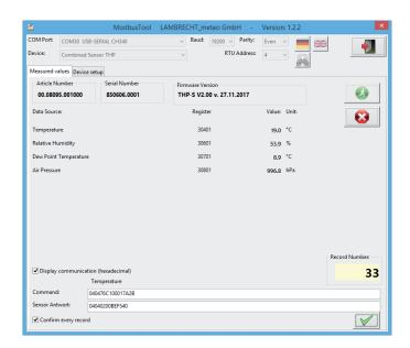
In the "Measured values" section, property data (article number, serial number and firmware version) and measured values are retrieved and displayed. In addition, the communication history can be displayed in hexadecimal format.
